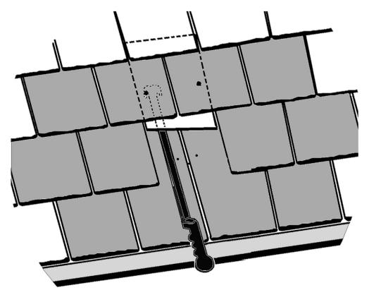
Slate ripper hooks slate nails and pulls them out, removing slate.
