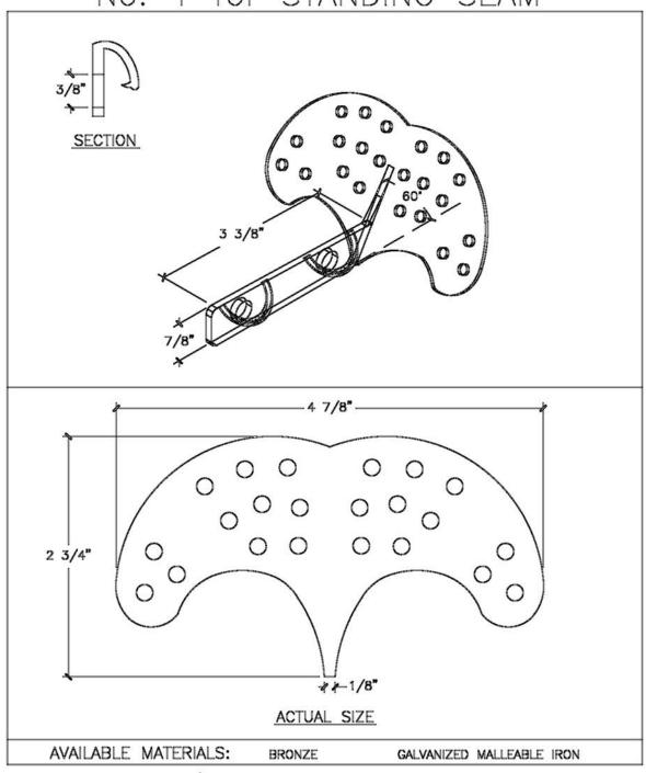
INFORMATION: THE ROOFER'S CHOICE SINCE 1883 FOR USE ON STANDING SEAM METAL ROOFS. THEY ARE PINCHED TO CLAMP ON THE TOP OF THE SEAM PROVIDING A RIGID PERMANENT JOB.
