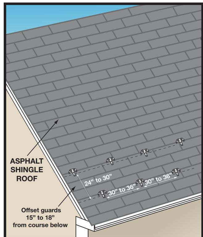
The patterns shown are typical for a rafter run of no more than 25 feet in an area with a ground snow load no more than 30 psf. If your project exceeds this criteria, contact Berger for a free consultation.
