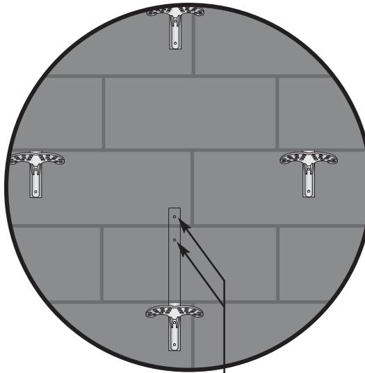
Nail Snow Guard here to secure to the roof.
